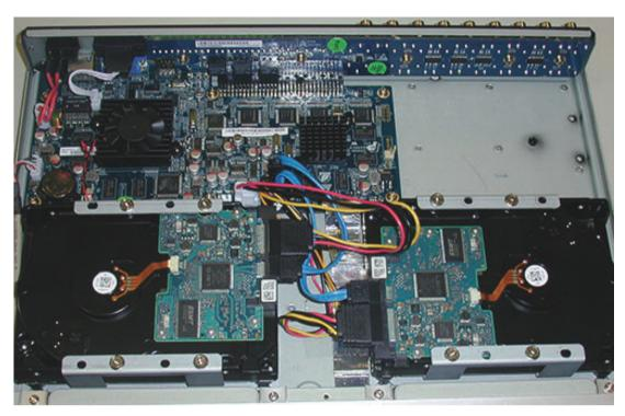
Figure 11.6: Install HDD 2 Use the same install steps described for installing HDD 1.
