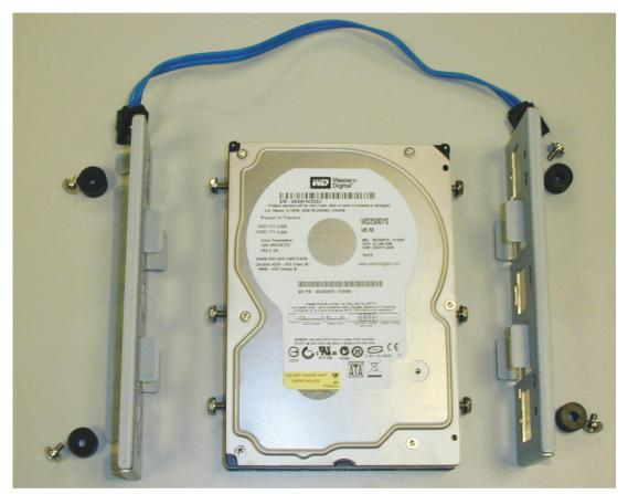
Figure 11.7: HDD install components (DIVAR 5000)
