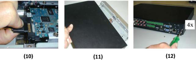
Figure 11.5: Install HDD 1
