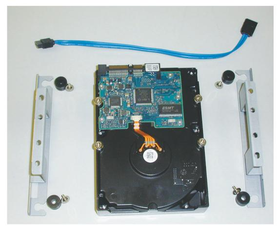
Figure 11.4: Install HDD 1 (DIVAR 3000)
