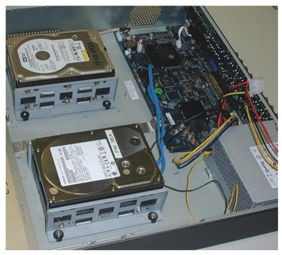
Figure 11.10: Install HDD 3 and 4
