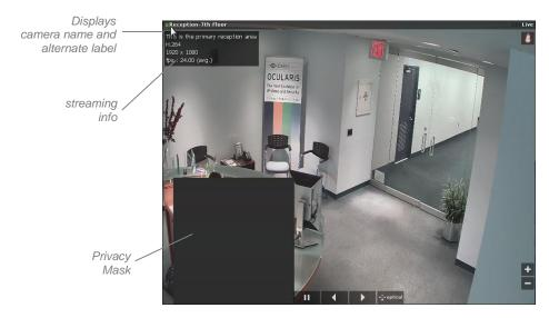
Additionally, if you position the mouse cursor over the block to the left of the camera name, you'll see a pop-up showing an optional description of the camera as well as other streaming information including the compression method, image size and frame rate of the camera shown.
