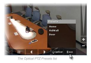
8. <u>Toggle between optical and digital PTZ</u>: Click the 'Optical PTZ' button to toggle between digital and optical PTZ.
