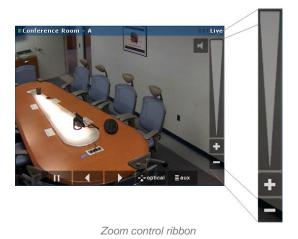
7. Optical PTZ presets: Click the 'aux' button alongside the playback controls to display the PTZ presets as configured on the recording component (see the individual recording component's user manual for more information). This will display the presets list.
