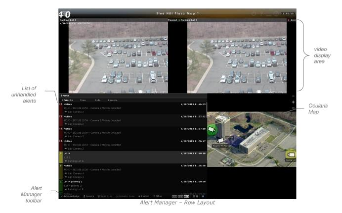
The Alert Manager screen may be customized between two layouts: 'Row layout' and 'Column Layout'. In 'Row Layout' (see example above), the upper section of the screen displays video related to the configured event that triggered the alert. The lower left section displays a list of alerts with associated information (event name, camera name, priority, timestamp, etc). The lower right section displays a map. If multiple maps are available, use the 'Locate' button to find the alert on a map.
