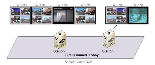
There is no technical limit to the number of screens/monitors which can encompass a video wall. There is, however, a limit to the number of screens that each Ocularis Client installation can support. Currently, each instance of Ocularis Client can support up to eight (8) monitors on a single station (or IP address). Therefore, if you wanted a video wall comprised of sixteen (16) monitors for instance, you would need at least two PCs, each with its own instance of Ocularis Client installed.
