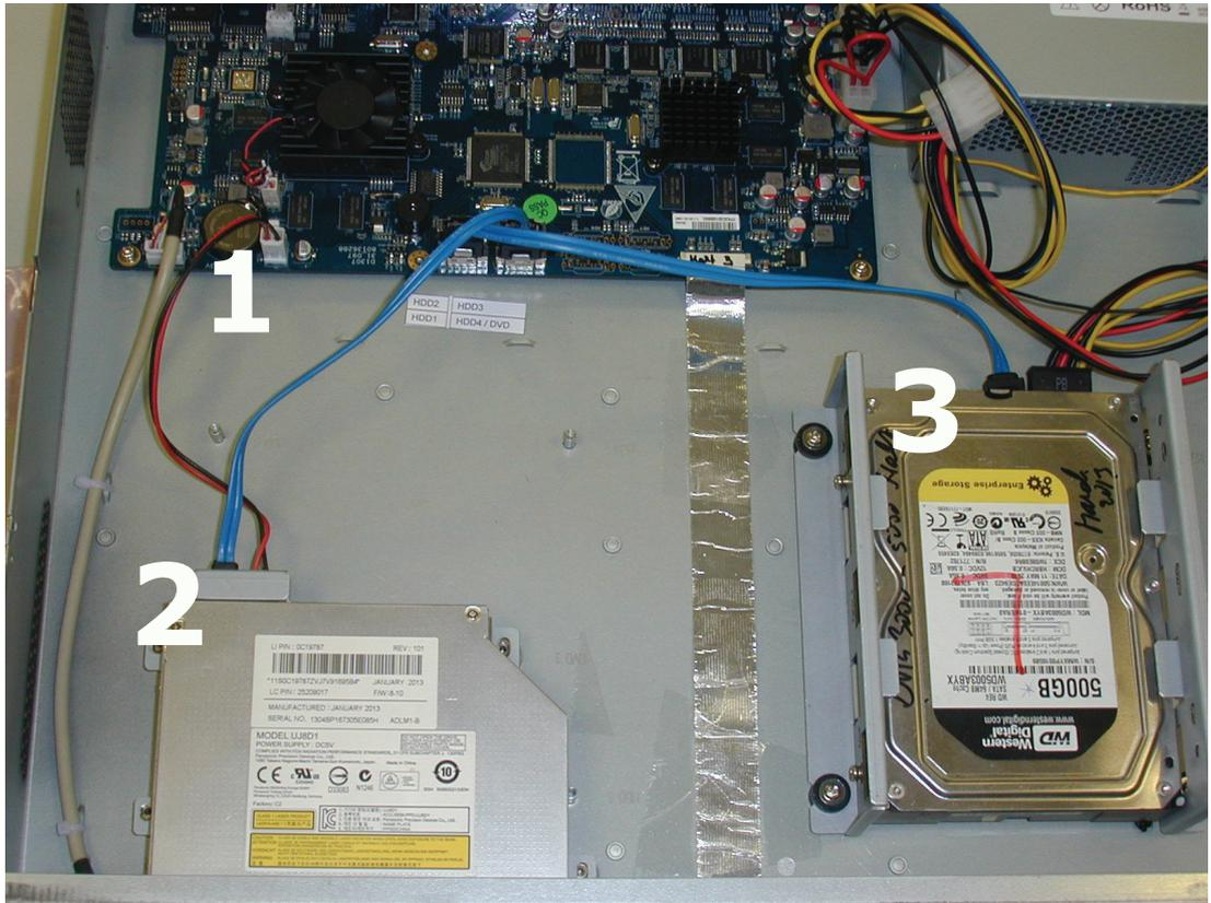
**Figure 11.2: DIVAR 5000 DVD and HDD installed**
