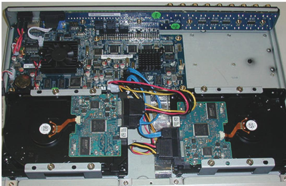
**Figure 11.6: Install HDD 2**
