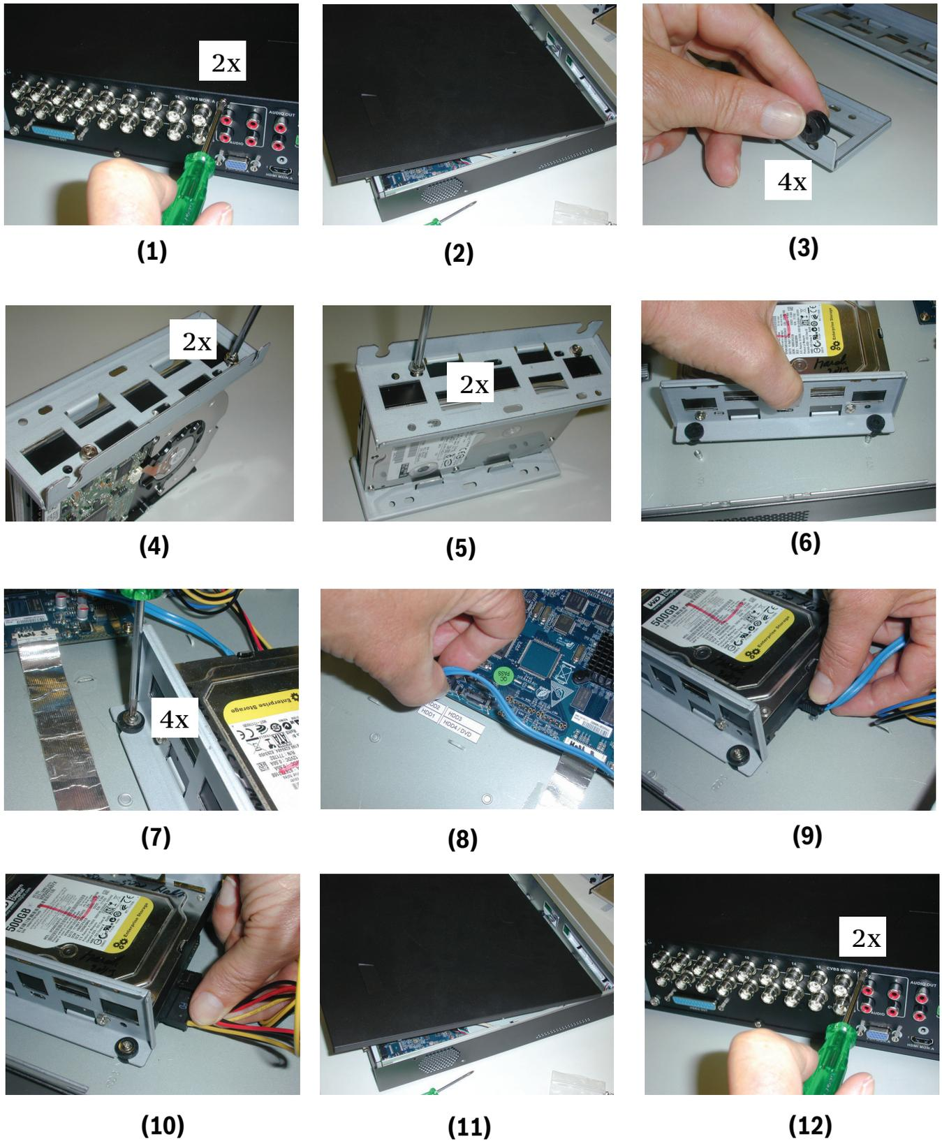
Figure 11.8: Install HDD 1
