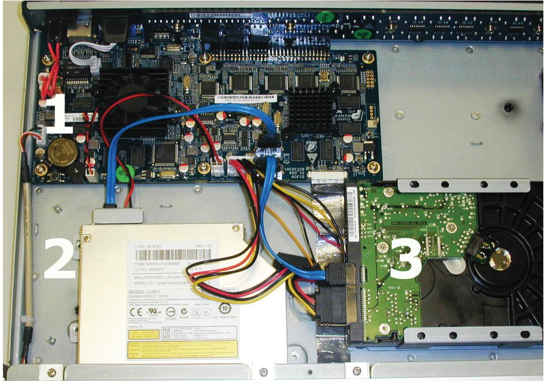
Figure 11.1: DIVAR 3000 HDD and DVD installed
