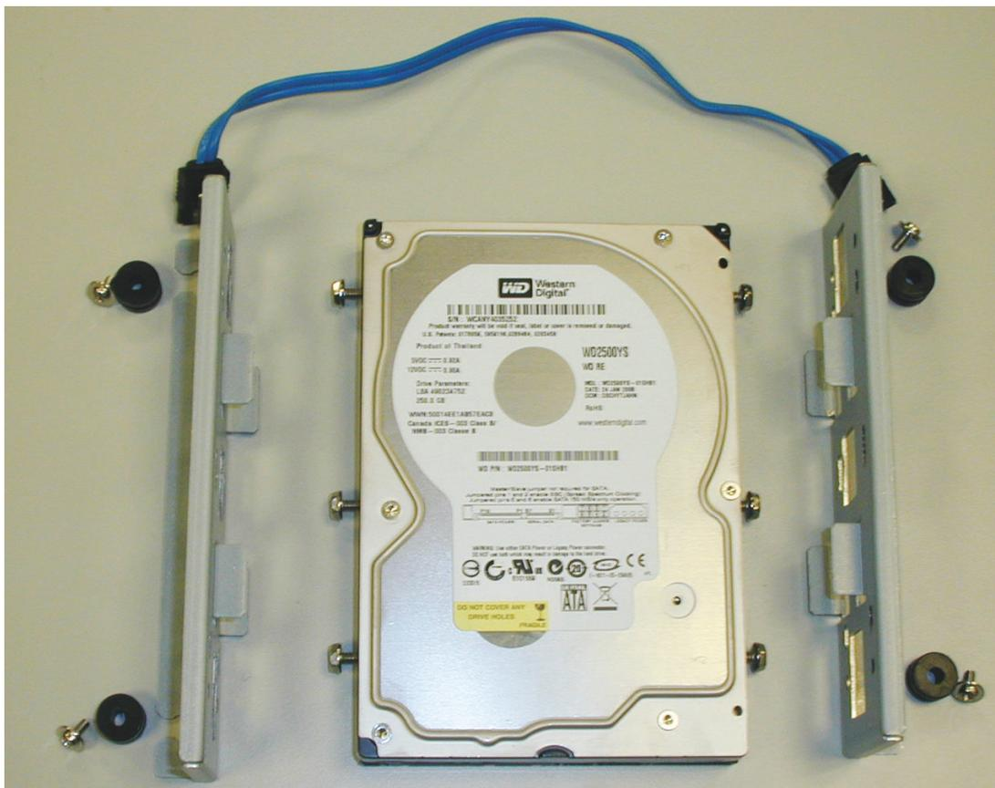
Figure 11.7: HDD install components (DIVAR 5000)
