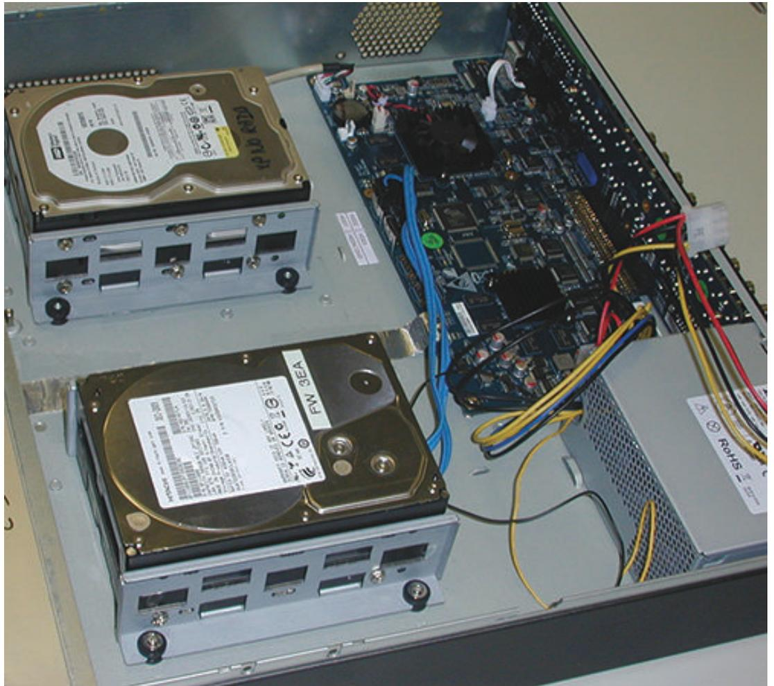
Figure 11.10: Install HDD 3 and 4
