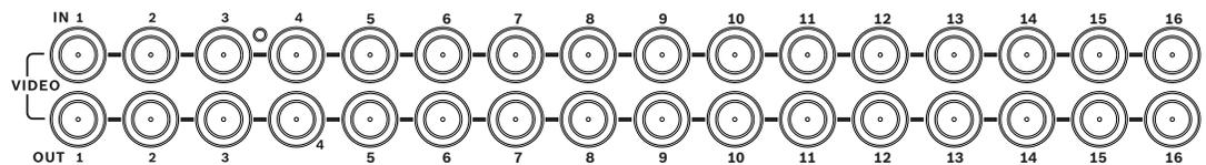
**Figure 4.1** 16 video inputs with loop-through outputs
