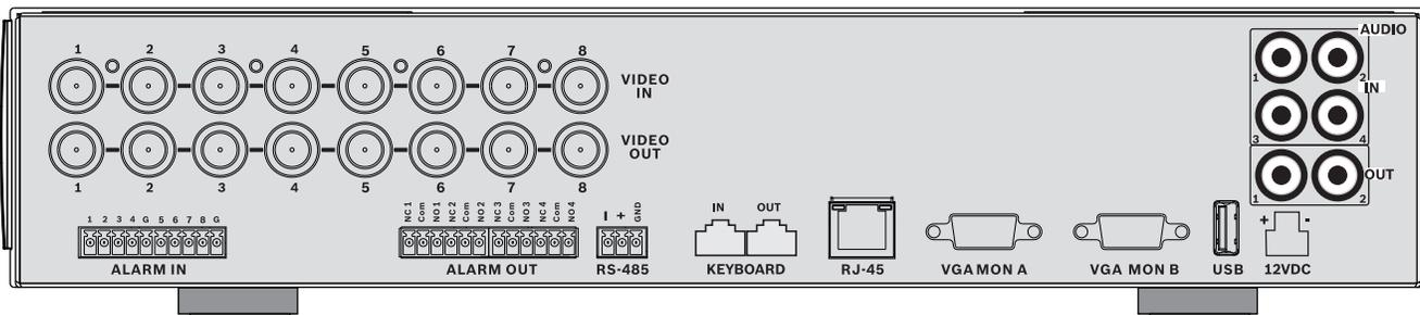
Figure 3.2 Back panel connections for 8-channel model
