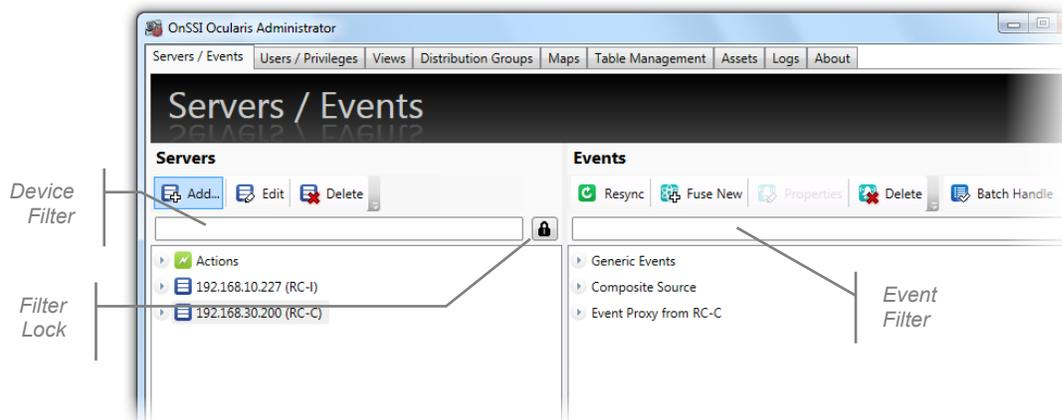
Figure 48 Device and Event Filters
