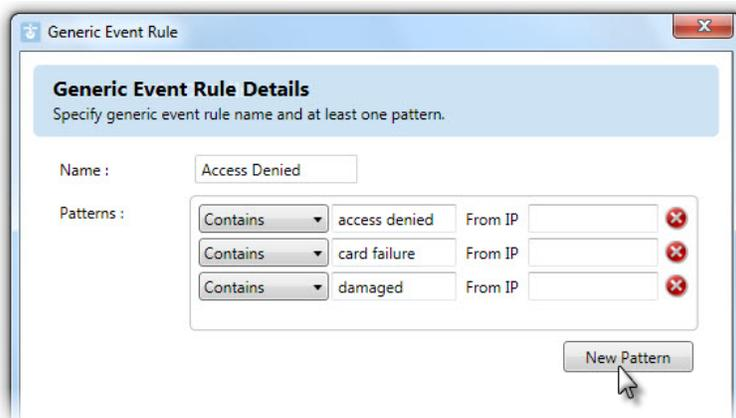
Figure 44 Using Multiple Patterns
