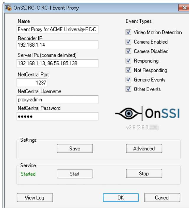
Figure 157 Sample RC-C Event Proxy configuration
