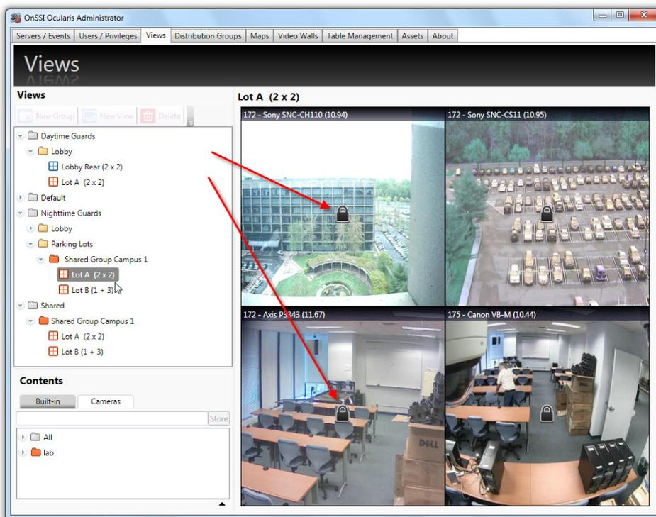
Figure 85 Padlock indicates view may not be modified in this selection
