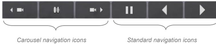
You can skip to the next and previous camera in the carousel sequence, as well as pausing the sequence. Once paused, the carousel will show the current camera indefinitely. To resume the carousel, click the checkmark icon.
