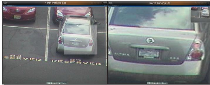
*Digital PTZ in live monitoring mode. Note the PIP window (upper right)*
