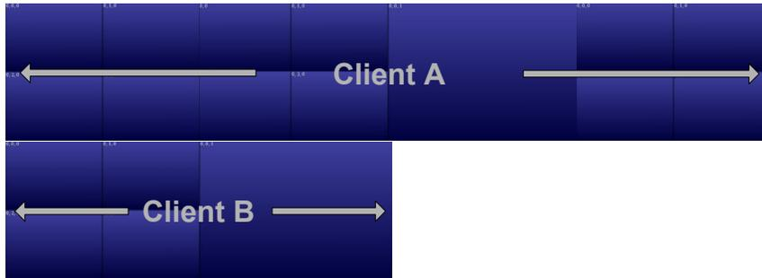
Four Screens from Client A on top of Two Screens from Client B (left justified)
